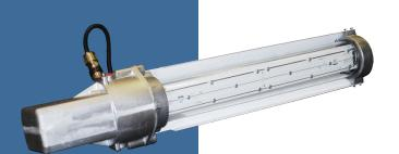
The **Lomond** is a rugged, flameproof LED luminaire. It features an integrated mounting channel for universal installation. The aluminium and glass construction make the Lomond highly resistant to aggressive chemical agents.
