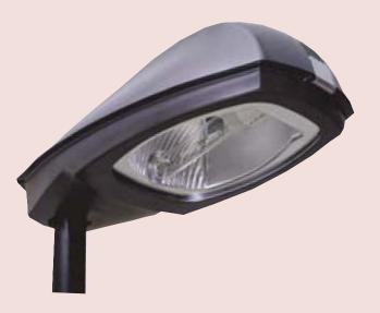
The Starline has a unique reflector system that provides optimum design spacing using 100-400W discharge lamps. The marine grade aluminium alloy body is suitable for use in coastal and harsh environments and the sealed optic system works effectively to keep out dust and dirt and maintain efficient roadway and perimeter lighting performance.
