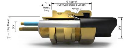
A robust and simple design for applications using SWA or AWA cable in a heavy industrial environment which is exposed to dust or extreme weather conditions. All cable glands can be supplied with a shroud, lock nut, serrated washer and an earth tag.
