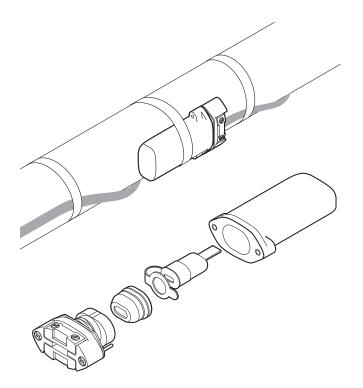
The nVent RAYCHEM E-150 is a cold applied low profile end seal. This universal end seal is designed to fit with all nVent RAYCHEM industrial self-regulating heating cables; BTV, QTVR, XTV and KTV meaning simplified product selection and reduced inventory to stock. It can be used in applications with temperatures ranging from  $-50^{\circ}\text{C}$  to 215°C. It is approved for use in hazardous areas.
