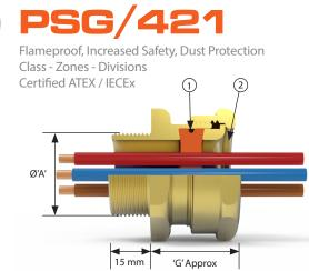
Unique pre-punched silicone barrier seal, provides (1)a barrier seal to individual cables, allowing multiple cables to enter through a single entry. No putty, resin or compound required to achieve an Exd flameproof barrier seal. Unused holes are to be fitted with the hole plugs provided
