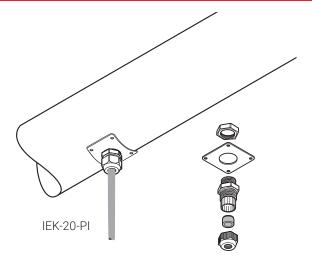
Insulation entry kits are designed to protect cables when passing through the thermal insulation cladding.
